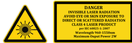
Output power and laser emission indicator label
